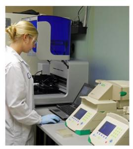
SIREM technician programing robot used to assemble Gene-Trac® qPCR reactions
